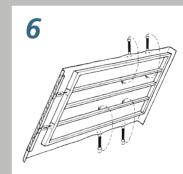
Tension tightly across the formwork using rubber hooks.
