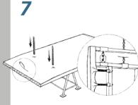
Cut crosses on the liner to mount lifting device and tie
