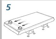
Tension the liner by turning the tensioning device.
